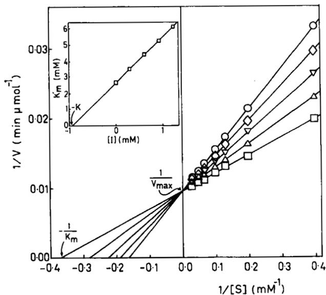
FIGURE 3 Double reciprocal Lineweaver-Burk plots for kinetics of jack bean urease at pH = 7.0 and T = 300°K in the presence of different fixed concentrations of sodium fluoride: 0 mM (□), 0.3 mM (△), 0.6 mM (▽), 0.9 mM (◇), and 1.2 mM (○). In the inset, a secondary plot of  $1/K_m$ -axis intercepts versus  $[I]$  is shown.
